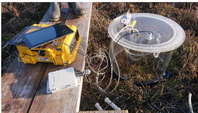
Typical GHG measurement equipment
